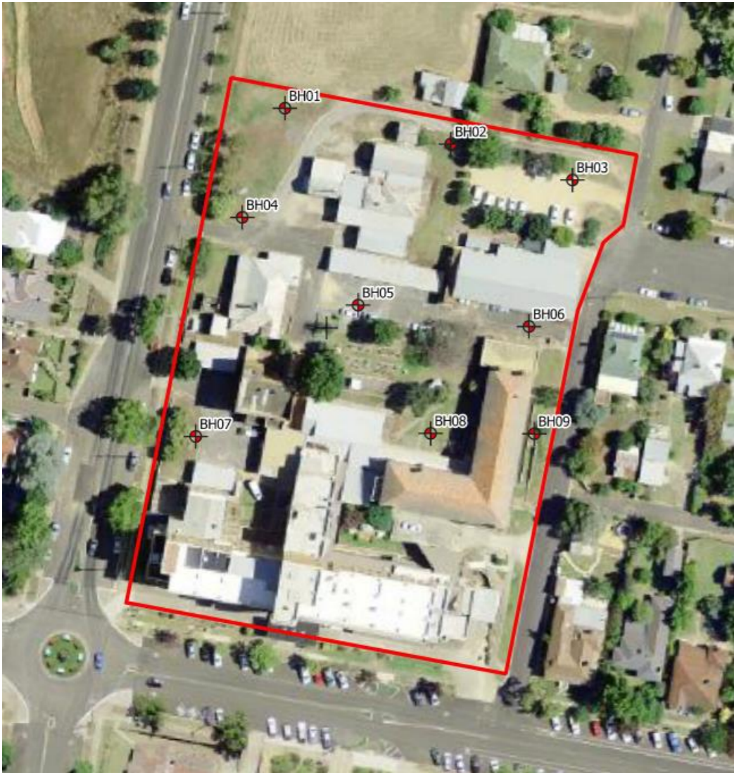
Figure 3 - Borehole locations (Source: Macquarie Geotech)
